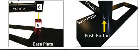
Base Plate Connections are made by holding the button down and sliding the red tube into the opposing tube on base until it locks in place.
