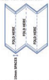
WHEN A GRAPHIC IS LARGER THAN STANDARD PANEL SIZE. FOLD FOR TRANSPORTATION AS SHOWN. THE PVC STRIPS MUST BE APPLIED WITH A 10MM GAP BETWEEN EACH LENGTH.
